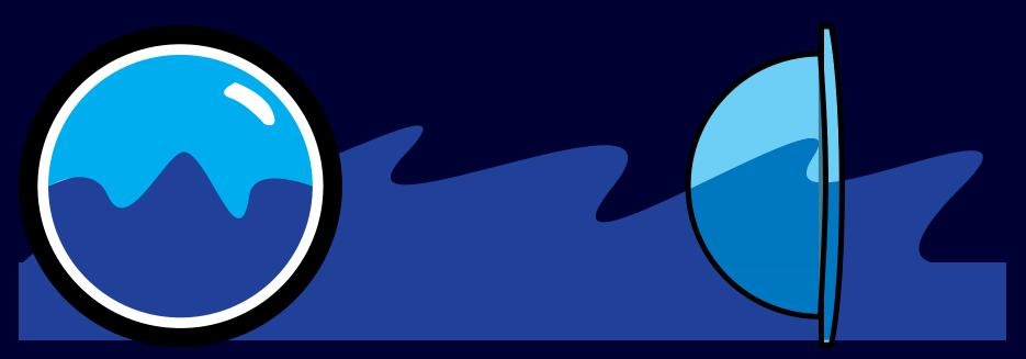
In a swimming pool or calm sea, the larger the dome, the less interruption there will be from water conditions. A preferred dome size would be around 100 mm in diameter or a 6-7 inch dome.
